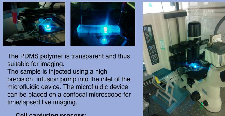
The PDMS polymer is transparent and thus suitable for imaging. The sample is injected using a high precision infusion pump into the inlet of the microfluidic device. The microfluidic device can be placed on a confocal microscope for time/lapsed live imaging.
