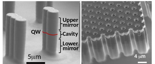
FIG. 1: Left: Two and three coupled micropillars. Right: honeycomb lattice of micropillars.
